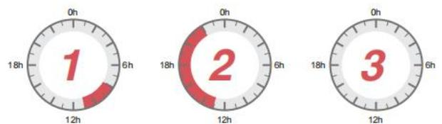
With 3 definable time periods, users can freely set the battery discharge time within the range of 00:00 to 23:59. During the time period set by the user, the inverter will give priority to the battery inverter to carry the load, and if the battery power is insufficient, the inverter will automatically switch to mains power to ensure stable operation of the load.
