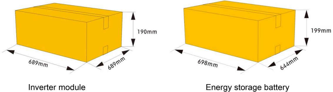
The energy storage battery module and Inverter module are packed in wooden cases with the size of 1120\*1400\*645mm, the number of packs is 10PCS, and the total weight is 400Kg.
