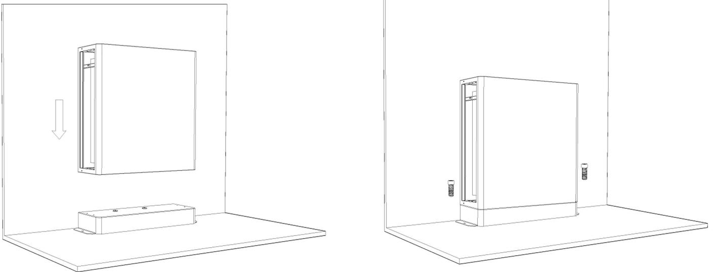
Install the second battery in the same way. After the installation is complete, install the wall fixing bracket.
