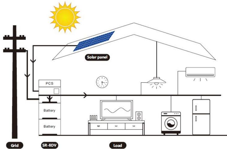
At night, the mains supplies power to the loads, and continues to charge the battery, if the battery is not fully charged.
